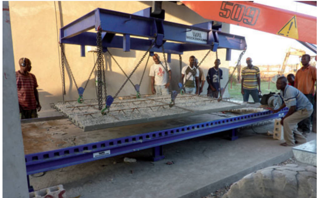
Precast flooring is produced on a stationary production table, provided by the German company Weckenmann (Images: Pro Haiti)
