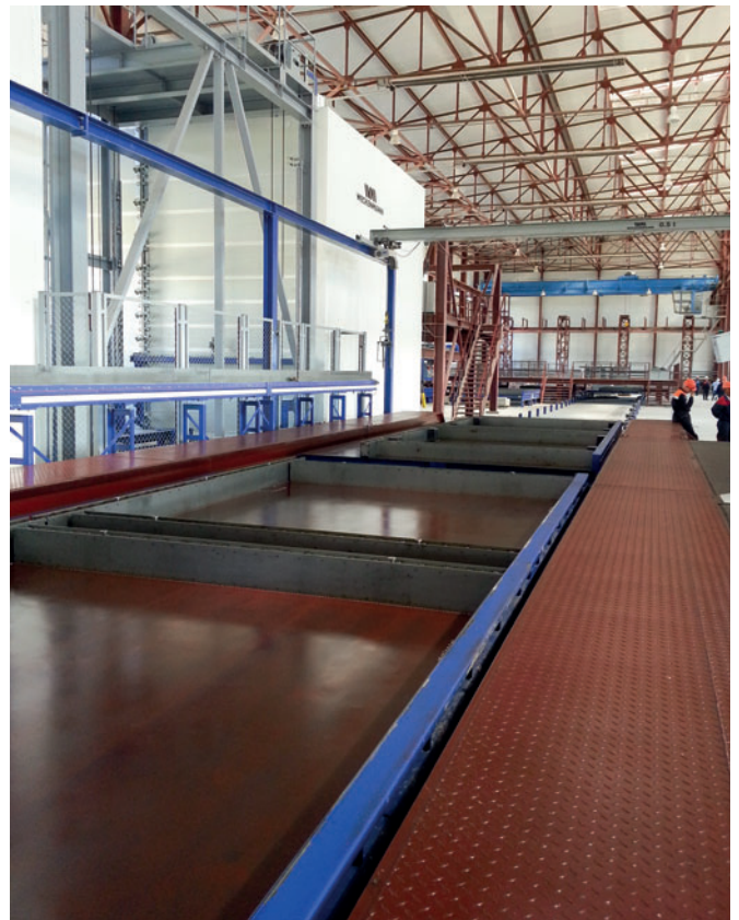
The new circulation plant that Weckenmann has erected in Kazakhstan is generously dimensioned for precast concrete elements.
