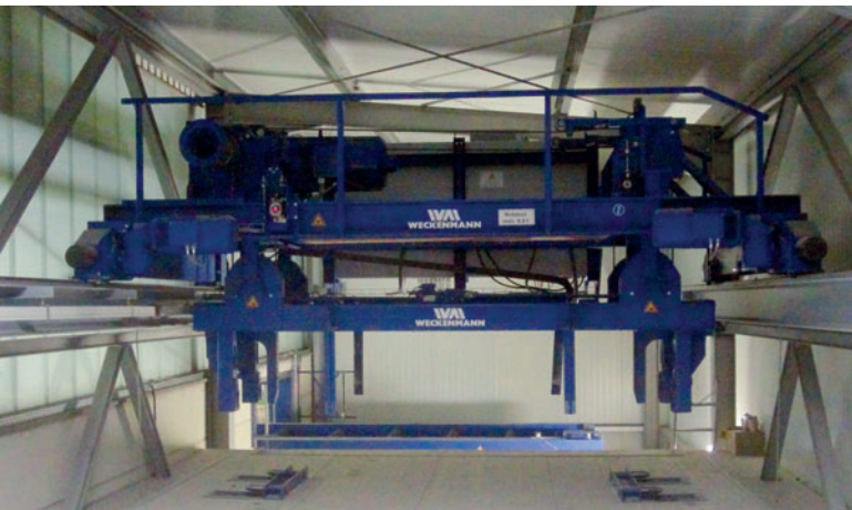
Fully automatic stacking crane
