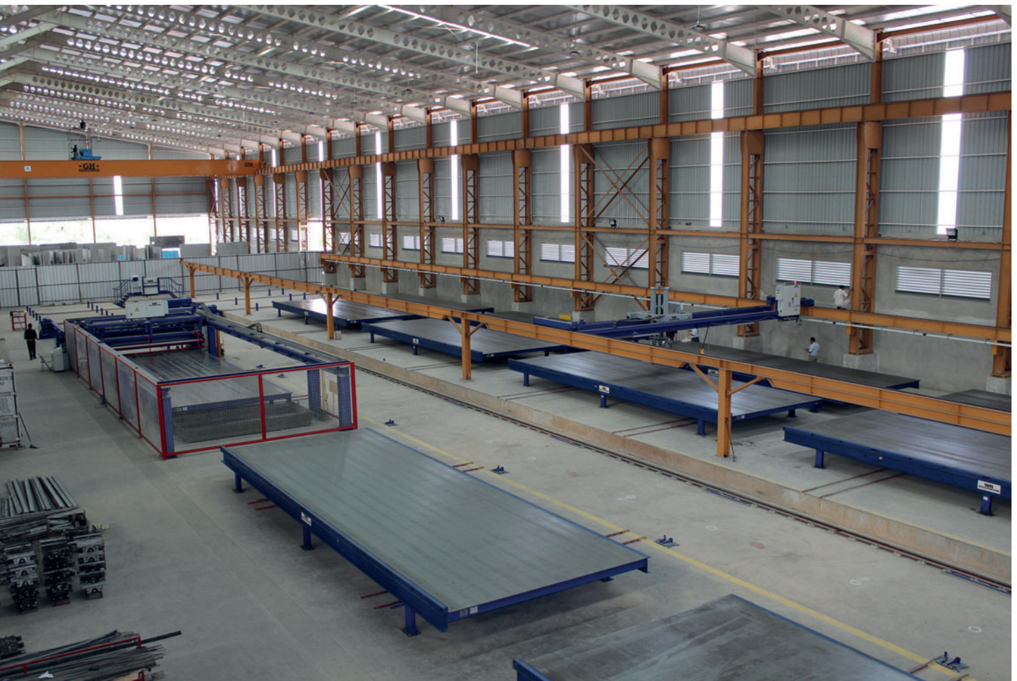
Central transfer table system
