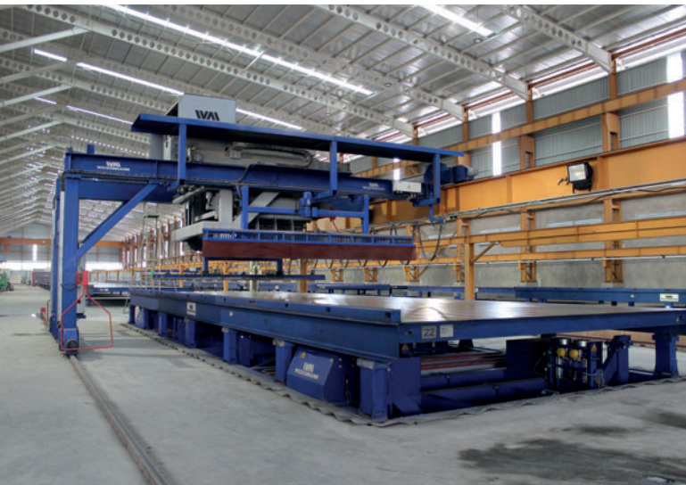
Concrete spreader with shuttering pallet and compaction station
