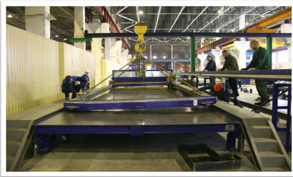
Pallet Circulation System with Prestressing Frame
