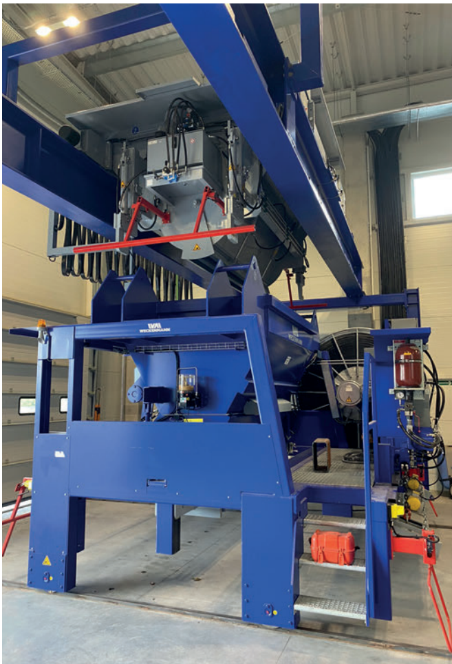
The concrete spreader
