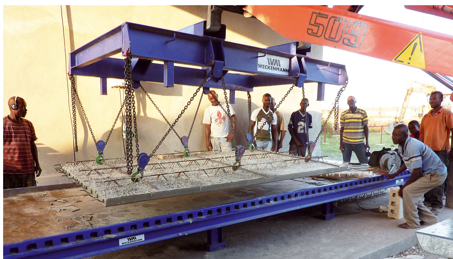
Precast floor slabs are produced on a stationary production table. (Picture: www.pro-haiti.de)
