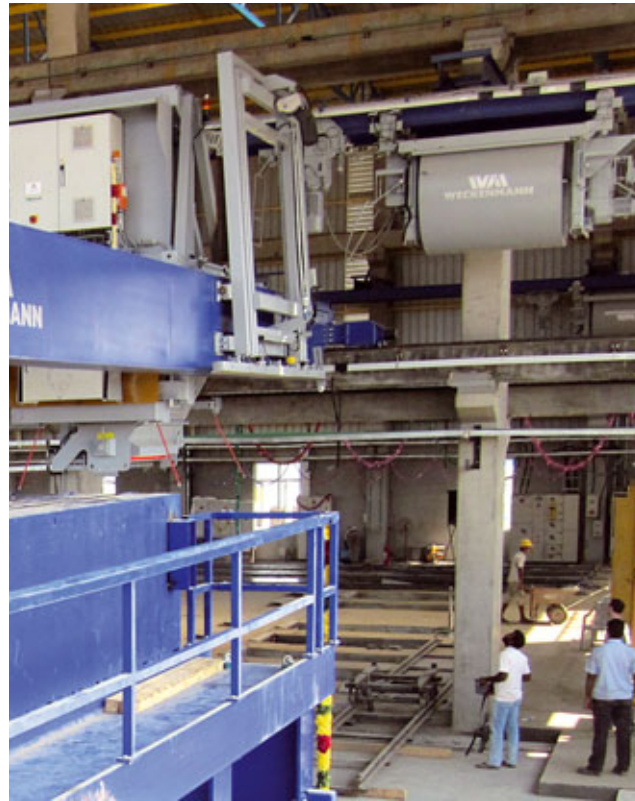
Whether single or double-rail system: Weckenmann bucket conveyor systems transport concrete quickly and safely to where it is needed in the production plant.
