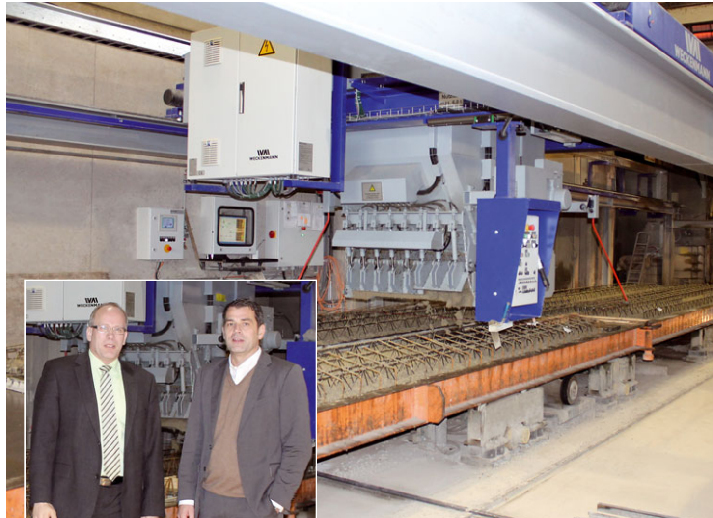
Managing director Thomas Beike (right) and technical project manager Benno Strack were able to optimise their processes and workflows with automatic concrete spreaders made by Weckenmann.
